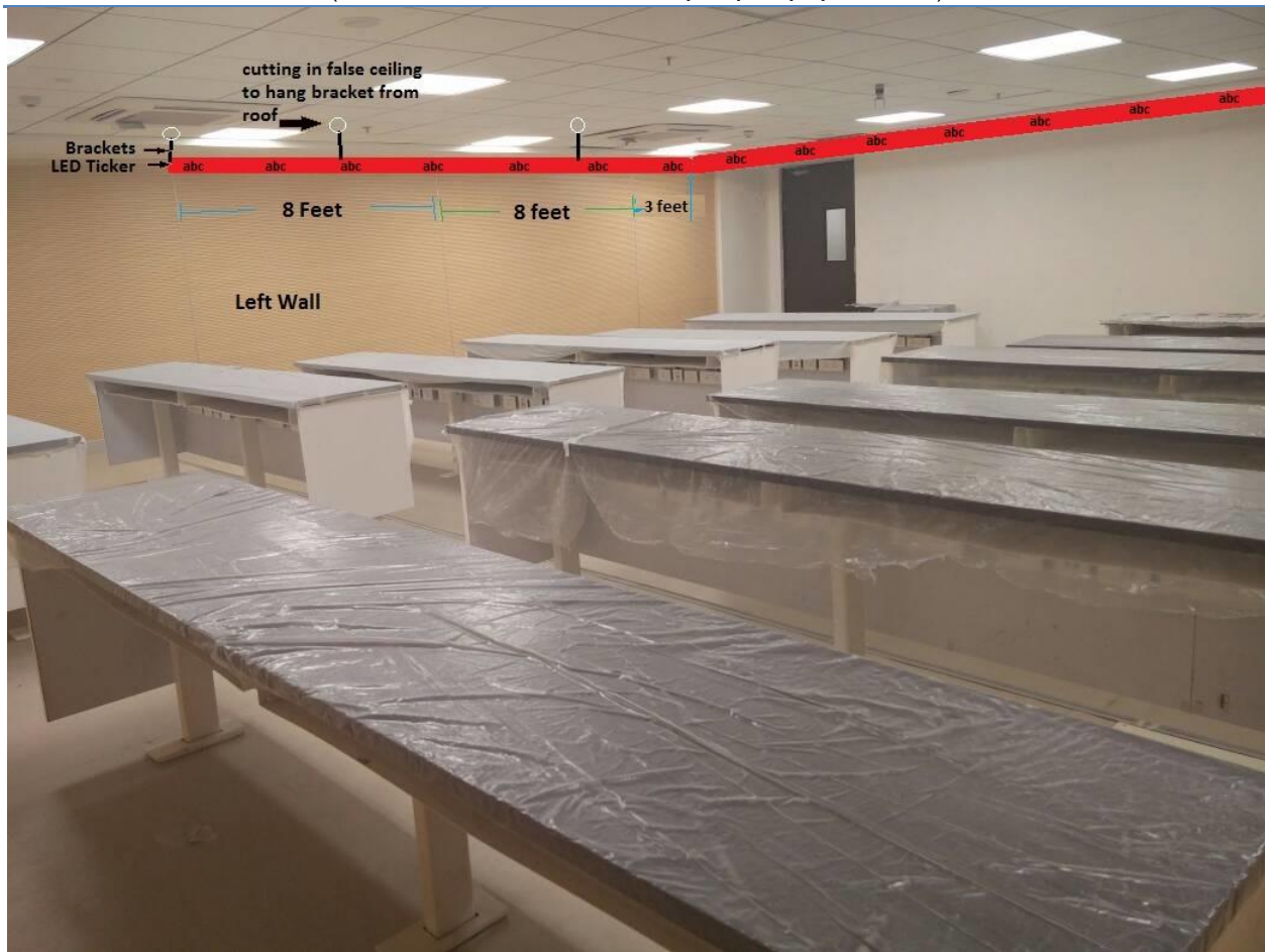
Picture 2: location of ticker display on the left wall of the Finance lab
